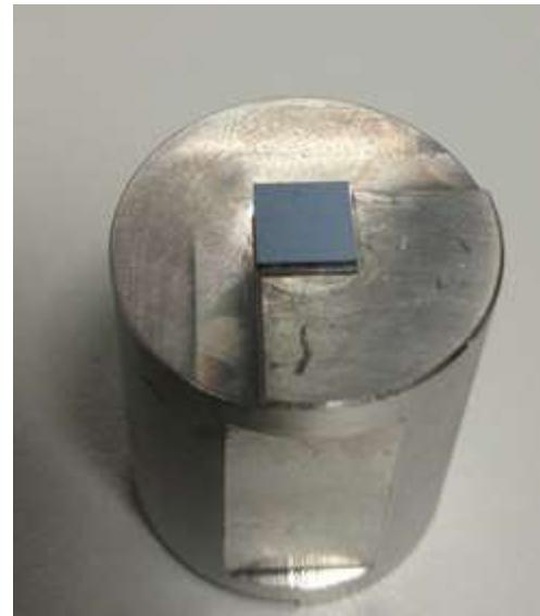
The measurement are conducted at **P23 beamline**, Energy 18 and 23 KeV, beam size  $VXH=3 \times 20 \mu\text{m}^2$ , sample size 5x5 mm, Different type substrates can be used, Pressure sensor available, Stepwise control of the pressure possible Working pressure: 1.6 - 80 MPa The liquid film is crated by drop-casting at the substrate.
