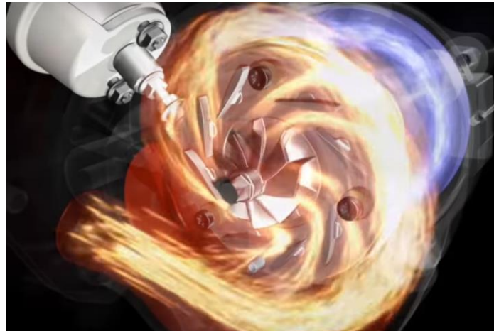
Variable vane geometry and wastegate mechanisms in Turbocharger
